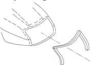
Step 2: Install the hardware: U-clamps, conic washers (in the upper holes), lower support (in the lower holes), hex bolts for the Flange nut, you should take a box end wrench to insert them between the light cover and the U-clamp. Tighten the nuts slightly.
