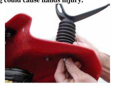
**NOTE**: To tight-fitting your light you will have to do a little 1/4" dia. (6.5mm) hole at the mark place in the bottom center of the windshield, then you won't have any problem to fit the light as you wanted.
