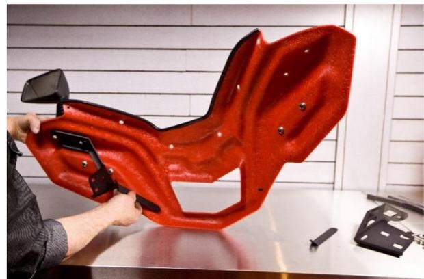
**Step 5:** Install the windscreen on color base using the 6 bolts 54-VIPA-1 with rubber washers & the 6 nuts 54-VIPA-2
