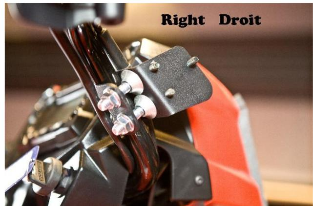
**Step 3:** Insert the 4 stainless steel bolts # 54-LNV-78 into the left and right mirror holes. Then turn the mirror base 180° (see Mirror Installation Guide).
